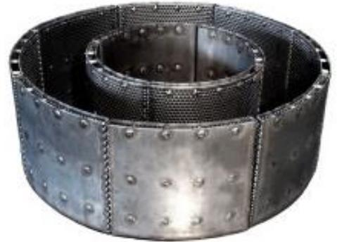
**Product Description** – Pellet Baskets made of Inconel sheet, custom perforated then fabricated to form 60 Degree radial section pockets
