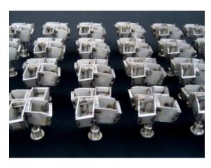
In this case, engine blades are coated at temperatures exceeding 1900 Deg F while exposed to a controlled atmosphere. Fixtures were designed to support / orient each blade for coating of the air foil while masking the root. Careful consideration had to be given to the effects of thermal cycling as well as the coating atmosphere.
