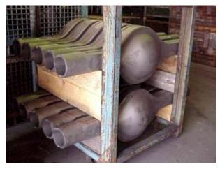
This was a difficult project due to three different weld specifications within the length of the assembly. Inconsistent fit up created a large challenge. While an optimal weld joint gap of 0.060" was appropriate, the actual gap ranged randomly from a max of .139" down to .010/" The parts were too thick / strong to reshape by merely using clamping within the robotic weld fixtures.
